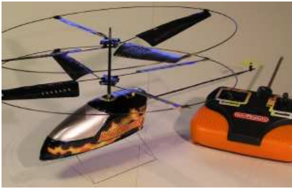
Bladerunner, 50 grams RC toy helicopter utilizing the Proxflyer rotor concept.
