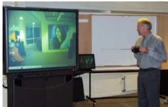
The Proxflyer Mosquito equipped with a wireless video camera is controlled solely by looking at a large video conferencing screen displaying the pictures coming from the helicopter.
