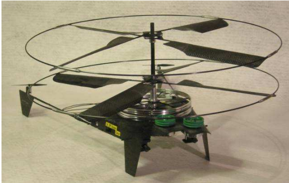
Fig.6 The Proxflyer MAV developed for the US Army to study stereo-vision operations.
